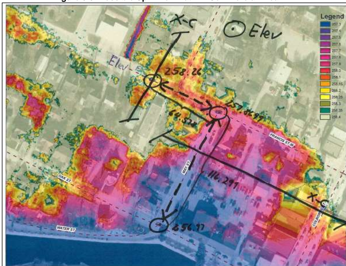
Figure 9.8: Possible Spill Flow Path in Commercial Area
