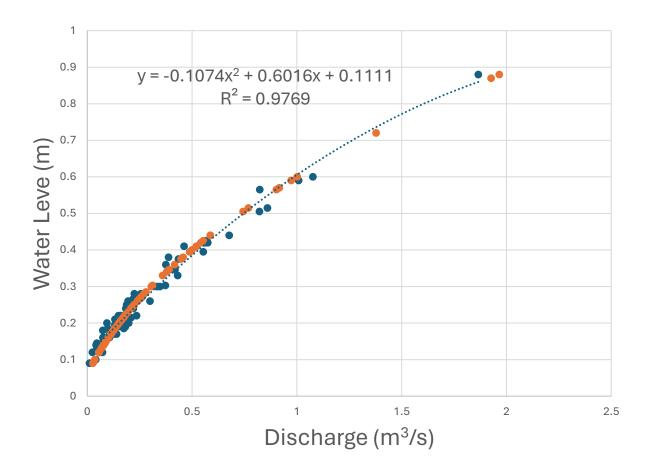
**Figure C.1**. Rating curve of Layton River at site SR2A from stage measurements (2009-2022).
