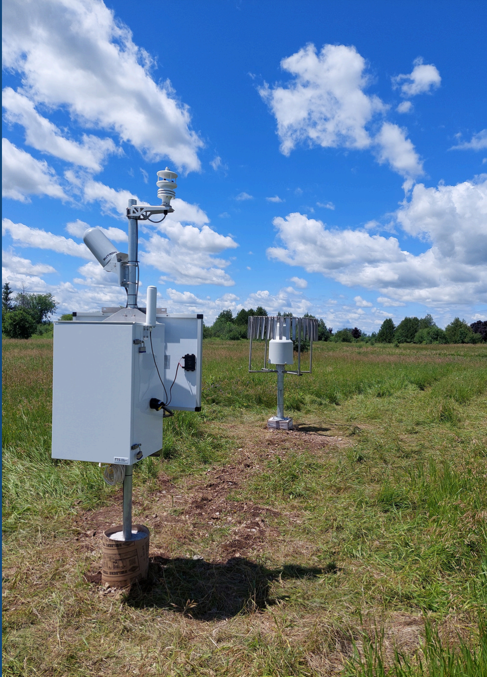
Weather Station at Ken Reid Conservation Area that monitors parameters such as precipitation, air temperature, relative humidity, and more.
