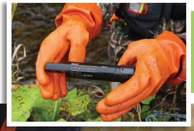
• We installed our first-ever conductivity logger at Blackstock Creek, which will track changes in dissolved salts in the water over time and give an indication of when contaminants might be entering the stream as seen by spikes in the data collected.
