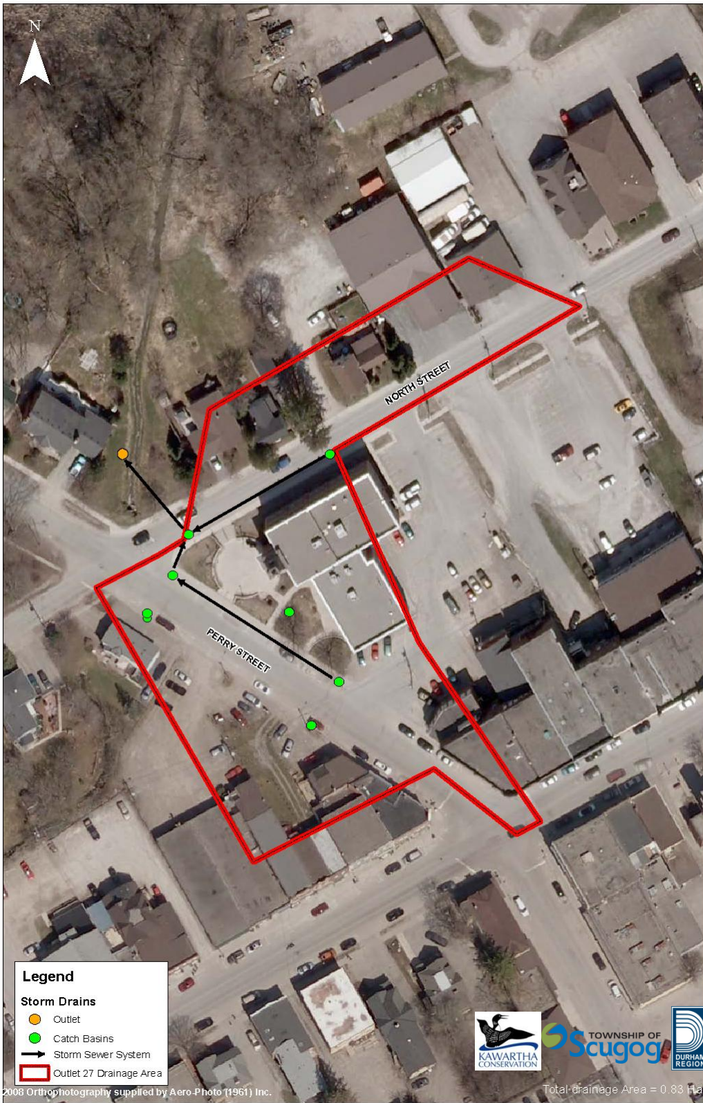
Perry Street Outlet 27 Storm Drainage Network
