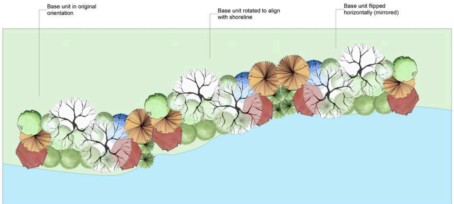
Figure 2: Base unit 5m by 2m arranged in different configurations to stretch the length of desired shoreline to be naturalized.
