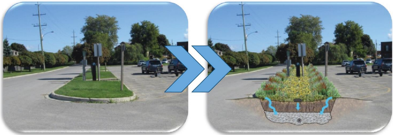
Figure 7 The Port Perry site shown above was chosen as the location for an urban demonstration site because large volumes of stormwater accumulate to this point, contributing to sedimentation into nearby Lake Scugog. The project demonstrates the Township of Scugog’s willingness to implement green infrastructure projects as an approach to water management – contributing to the restoration of the natural water cycle and a more resilient community.
