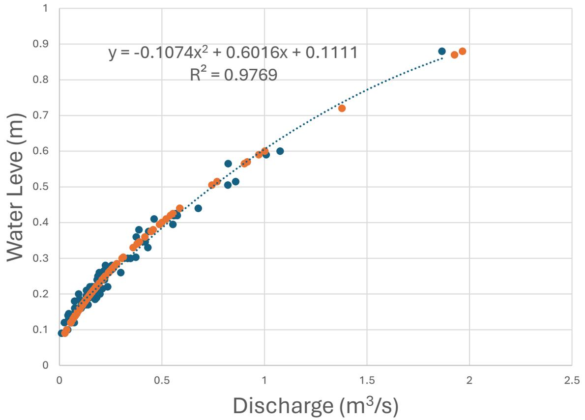
**Figure C.1.** Rating curve of Layton River at site SR2A from stage measurements (2009-2022).
