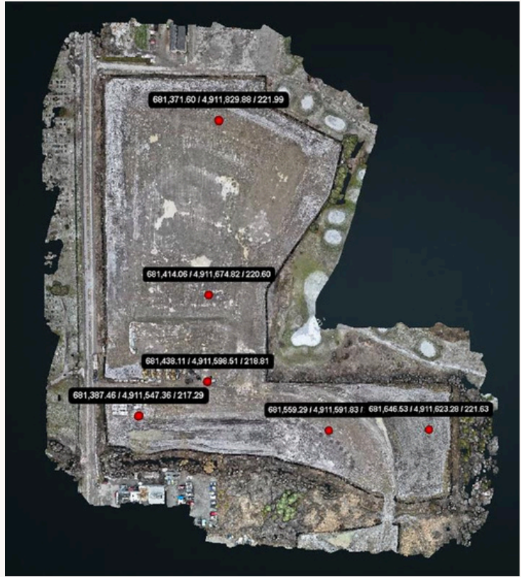
Aerial drone image of site, with locations of ground control points.
